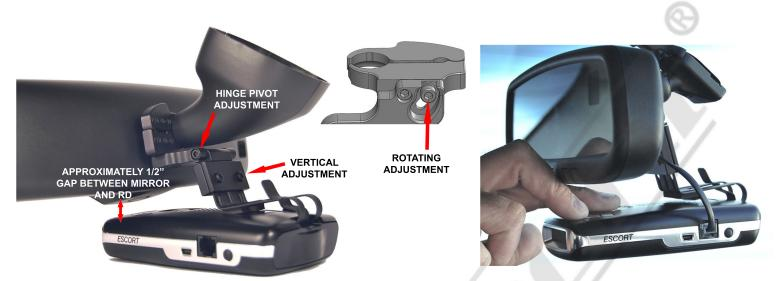
5 - Install the RD onto the mount. Make the necessary adjustments as shown above. Using the vertical adjustment, we recommend you adjust the RD so there is approximately 1/2" gap between the bottom of the mirror and the top of the RD. After all adjustments are made, be sure to check that all adjustment screws are tight. Grab the long arm of the allen wrench to assure that these screws are securely tightened. You will not strip out the tapped holes in the aircraft grade aluminum.
