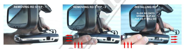
7 - When removing or installing the RD, squeeze the trigger and the back side of the mount together with one hand, and lift the front of the RD upward with the other hand before sliding the RD off or onto the spring clip. You must lift the front of the RD upward before sliding it off or onto the mount.
